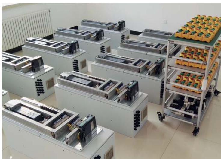
Electrical Control Cabinet 电控柜
