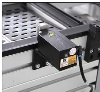
BU.PN.02/A-60 installed at the joint of the conveyor. It is used to buffer and stop the pallet infeeding or outfeeding from the main conveyor. BU.PN.02/A-60安装于线体对接处，用于缓冲并挡停移入移出主线体的托盘
