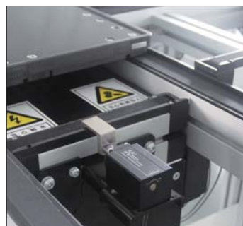
BU.PN.02/B-60 installed on the Lift and Transverse Unit(3 position) at the joint of the conveyor. It is used to buffer and stop the pallet outfeeding from the main conveyor. BU.PN.02/B-60安装于线体对接处的3位置顶升横移上，用于缓冲并挡停移入移出主线体的托盘
